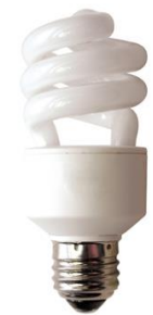
A CFL contains a mixture of argon and mercury gases that produces invisible ultraviolet light (UV) when the gas is excited by electricity.
