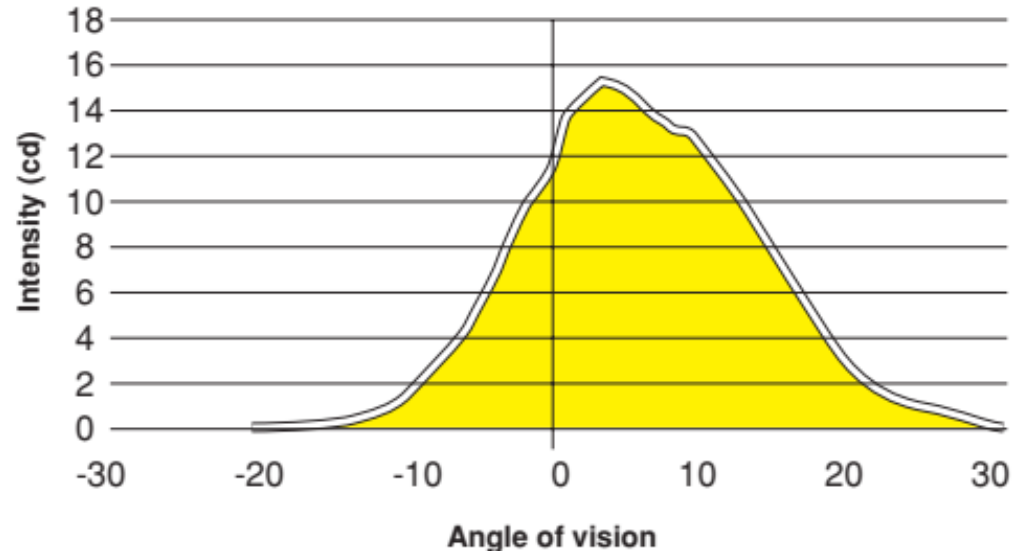
Sign beacon with amber-coloured LED
